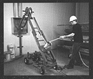
THE ULTRA BRUTUS™ Collaboration between our Industrial and Electrical segments resulted in the innovative Ultra Brutus™ cable puller – improving safety and increasing productivity for end users. Gardner Bender engineers utilized hydraulic cylinders made by Milwaukee Cylinder to turn what was nearly an hour long set-up job for two electricians into a two minute task for one.
