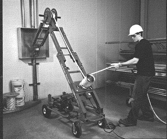
**THE ULTRA BRUTUS™** Collaboration between our Industrial and Electrical segments resulted in the innovative Ultra Brutus™ cable puller – improving safety and increasing productivity for end users. Gardner Bender engineers utilized hydraulic cylinders made by Milwaukee Cylinder to turn what was nearly an hour long set-up job for two electricians into a two minute task for one.
